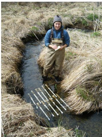
Left: grad student, Pam Kostka, with installed array for measuring instream periphyton growth in one of the headwater streams. Right: Crew collecting groundwater samples from wells along alder flowpaths.
